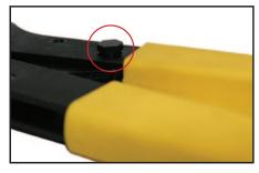
4. Push the adjuster cam out from the circlip side until the hexagon head of the cam disengages from the handle, and turn the cam anticlockwise, so that it is moved around I flat of the hexagon.
