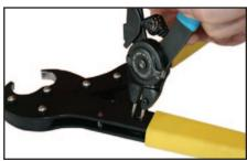
2. Turn the tool over and remove the circlip securing the adjuster cam.
