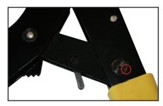
I. Identify the position of the adjuster cam by locating the dot on the hexagonal end of the cam.
