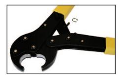
3. Retain the circlip for replacement after adjustment.
